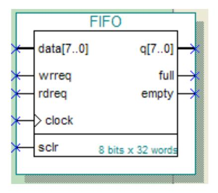
module FIFO ( clock, data, rdreg, sclr, wrreg, empty, full, q); input clock; [7:0] data; input input rdreg; sclr; input input wrreg; output empty; output full; output [7:0] q;
